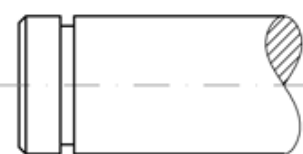
Groove rolled the snap ring
